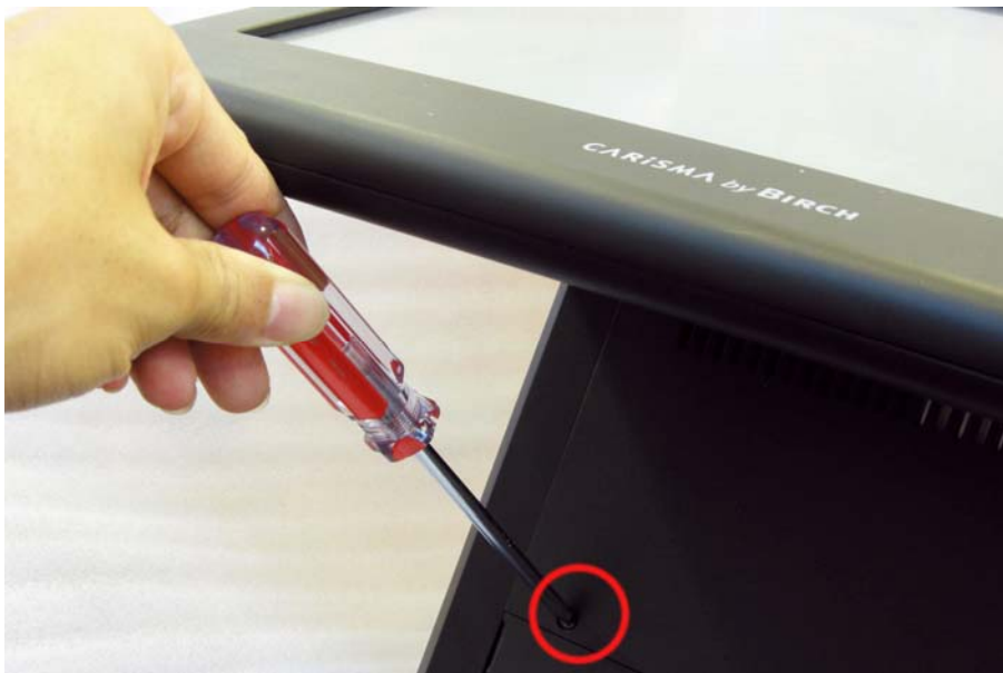
3. After changing RAM module, please lock the four screws for front housing
