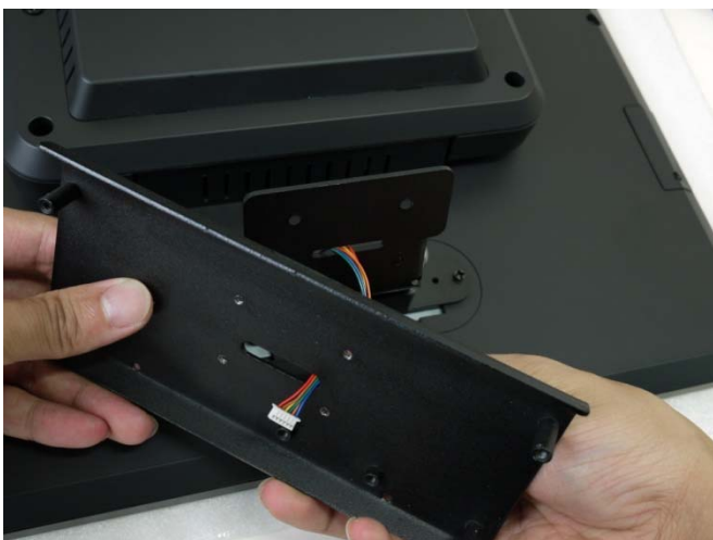
10. Pass the signal line through the middle of the VFD base
