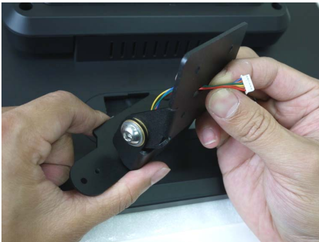
8. Pass the signal line through the middle of the upper of hinge mount hole
